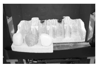
c) Place the right hand front pebble rail moulding onto the front ceramic rail support and locating pins as shown below in Fig. 12
